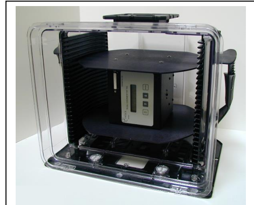
Figure 1 - Vib Tool mounted in 300 mm FOUP
