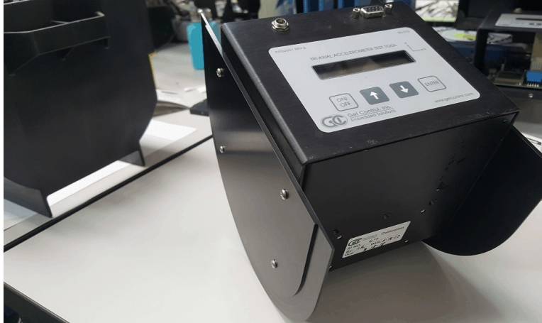
Figure 7 - 200 mm Plates Mounted on Vib Tool
