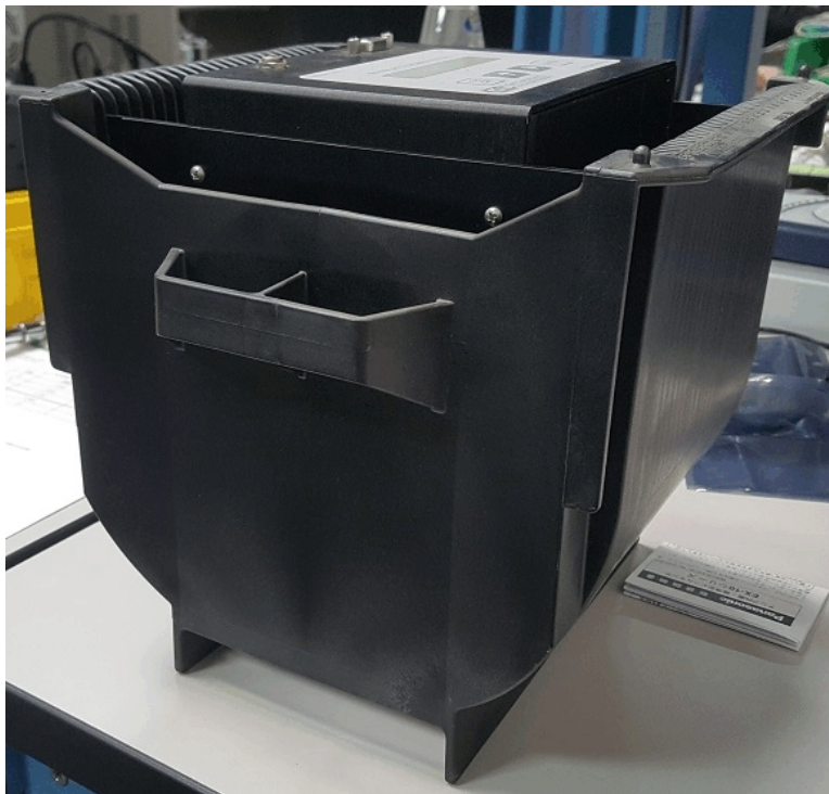
Figure 8 - Vib Tool Installed in 200 mm Carrier
